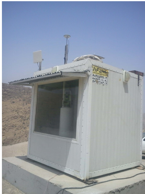
Figure 2: location of TPSR site with its sensors, GPS/GLONASS antenna on top of the room and TPS inside the room on the pillar
