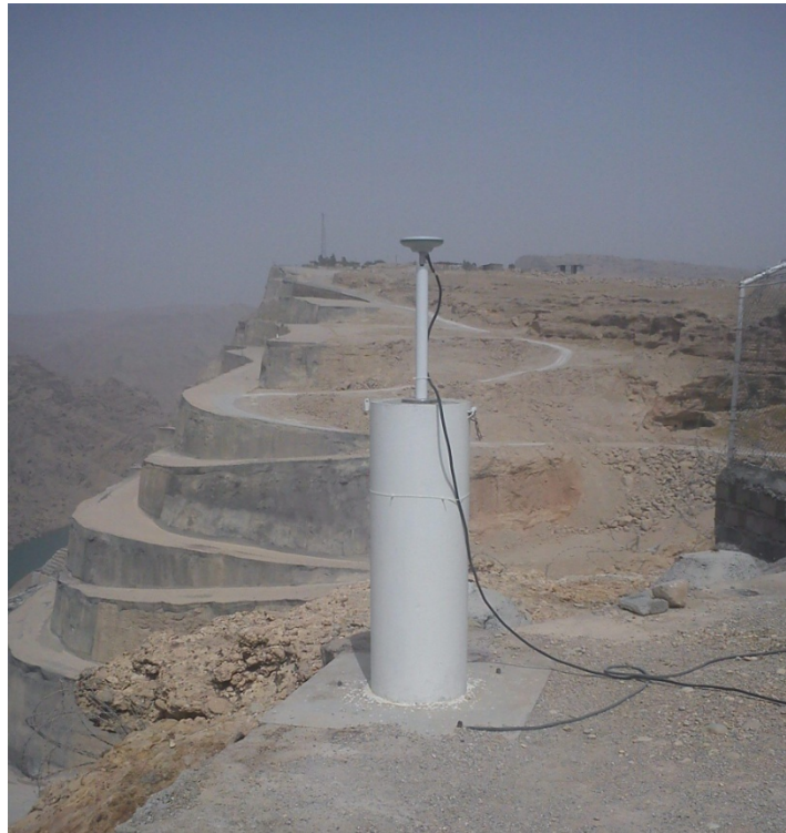
Figure 3: location of GPSR site, GPS/GLONASS antenna on top of the pillar
